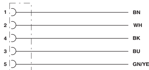
Contact assignment of the M12 sockets
