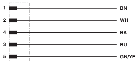
Contact assignment of the M12 plug
