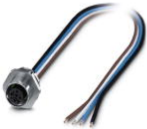
Bus system flat-type plug, PROFINET, 4-position, SocketLink:M12, D-coded, Front mounting, M16 x 1.5, Individual wires, Cable length: 0.5 m
