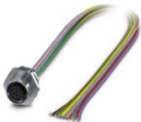
Flush-type connector, Universal, 17-position, SocketLink:M12, A-coded, Front mounting, M16 x 1.5, Individual wires, Cable length: 0.5 m
