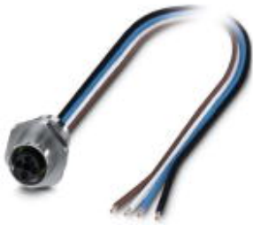
Flush-type connector, Power, 4-position, SocketLink:M12, T power, Front mounting, M16 x 1.5, Individual wires, Cable length: 0.5 m
