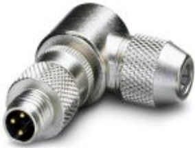
Connector, 3-position, shielded, Plug angled M8, A-coded, Solder connection, Knurl material: Nickel-plated brass, External cable diameter 3.5 mm ... 5 mm
