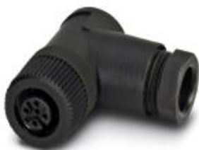
Connector, 5-position, Socket angled M12, A-coded, Screw connection, Knurl material: Plastic, Cable gland Pg9, External cable diameter 6 mm ... 8 mm
