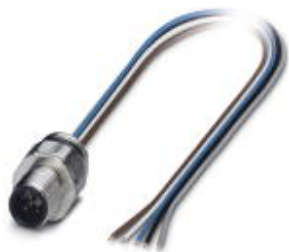
Sensor/Actuator flush-type plug, 5-pos., M12, A-coded, front/screw mounting with Pg9 thread, can be positioned, with 0.5 m TPE litz wire, 5 x 0.34 mm 2
