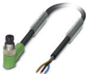
Sensor/Actuator cable, 3-position, PUR halogen-free, black-gray RAL 7021, Plug angled M8, on free cable end, Cable length: 10 m
