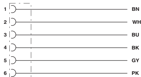
Contact assignment of M8 socket
