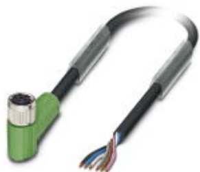
Sensor/Actuator cable, 6-position, PUR halogen-free, black-gray RAL 7021, free cable end, on Socket angled M8, Cable length: 5 m
