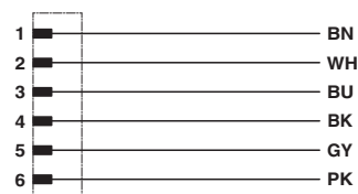
Contact assignment of the M8 plug
