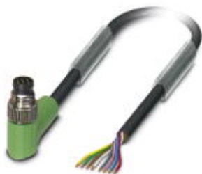
Sensor/Actuator cable, 8-position, PUR halogen-free, black RAL 9005, Plug angled M8, on free cable end, Cable length: 5 m
