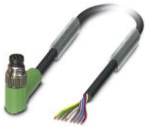
Sensor/Actuator cable, 8-position, PUR halogen-free, black RAL 9005, Plug angled M8, on free cable end, Cable length: 10 m
