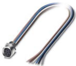
Sensor/actuator flush-type socket, 6-pos., M8, front/screw mounting with M8 fastening thread, with 0.5 m TPE litz wire, 6 x 0.14 mm 2
