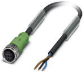
Sensor/Actuator cable, 3-position, PUR halogen-free, black-gray RAL 7021, free cable end, on Socket straight M12, A-coded, Cable length: 5 m
