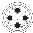
Connector pin assignment of M12 plug, 4-pos., S-coded, view of pin side
