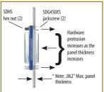
"Note: Maximum recommended panel thickness is 0.062". Dimensions in excess of 0.062" can limit proper cable mating due to hex nut protrusion. Panels that exceed 0.062" can be milled down to the recommended thickness in the area around the adapter.
