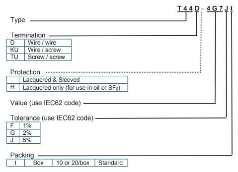
Note: Standard TCR is 100ppm/°C. Contact factory for 50 and 25ppm/°C grades.
