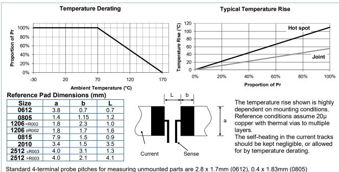
0.4 x 2.8mm (1206), 1.2 x 4.5mm (2010) and 1.5 x 5.8mm (2512). All probe location tolerances ±0.02mm.
