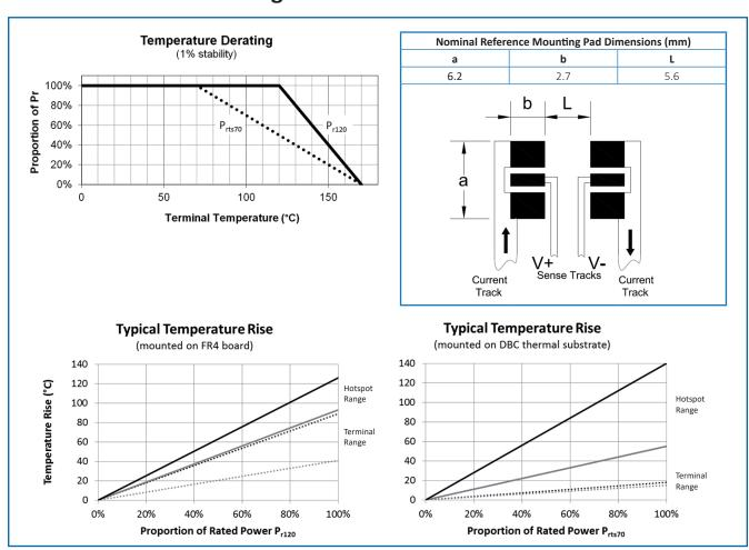
FR4 board details: 102x51mm, high  $T_g$  FR4 board with  $70\mu m$  (2 ounce) inner and outer Cu planes or similar substrate, such that terminal temperature is maintained at  $\leq 120$ °C.
