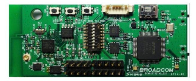
The Cypress WICED<sup>™</sup> Smart BCM92073X\_LE\_Kit ("Tag3") is an evaluation board that exposes various pins on the BCM2073X BLE SoC device family for debug, evaluation, and troubleshooting. The BCM2703X BLE SoC family offers Bluetooth Low Energy (BLE)-compliant, stand-alone baseband processors with integrated 2.4 GHz transceivers.
