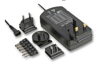
This plug top switch mode power supply provides a choice of 20 fully regulated output voltages. The voltage cannot be changed by mistake by the end user as there is no selector switch. The voltage is chosen by way of a resistor which pushes into side of the power supply. The table below shows the complete choice of outputs which step up in 1vdc increments and range between 5vdc and 24vdc
