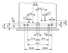
Fixation on PCB or housing from below
