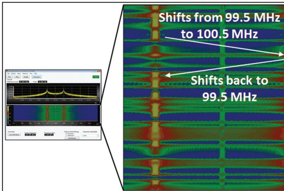
A closer look at a spectrogram display reveals more detail on the actual frequency shift keying between the two frequencies as a function of the PN data sequence being used to control the frequency shift keying.
