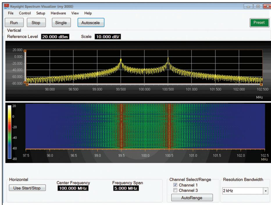
The top plot in Figure 1 is a frequency spectrum measurement with amplitude (dBm) on the y-axis and frequency (MHz) on the x-axis. We can see that the FSK signal is shifting between the two frequencies, by observing the two peaks on the frequency spectrum. The center frequency, frequency span, and resolution bandwidth have been set to measure the 100 MHz carrier which is being FSK-modulated between two frequencies, 99.5 MHz and 100.5 MHz ( $\Delta F = 1$  MHz).
