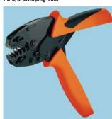
A crimp tool for ferrules to DIN 46228 part 1 and 4 with and without plastic collars from 0.25 to 6mm² (AWG24...10). Five crimping profiles for the rated conductor
