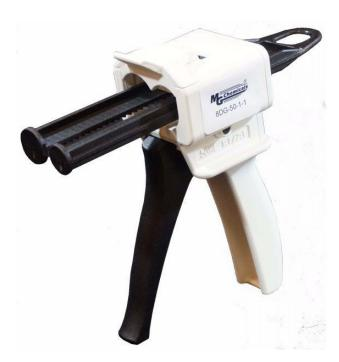
The 8DG-50-1-1 is a dispensing gun, made of solid plastic, for use with dual cartridge systems. It features an easy snap in / snap out cartridge insertion system that facilitates cartridge installation in seconds. The trigger activated control provides a steady increment flow of hardener and resin through an optional static mixer that can be attached to the head of the cartridge. Simply pull the trigger and obtain exactly mix ratio of material needed to complete your task.
