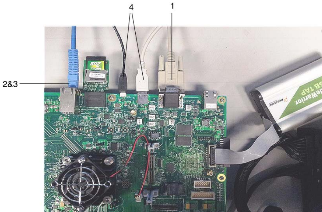
Figure 14. T2080QDS board connections
