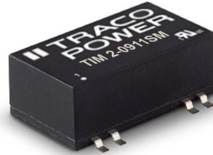
The TIM 2 series is a range of high performance, regulated 2 Watt DC/DC converters in a DIP-16 plastic package. The reinforced I/O-isolation system complies with the medical safety requirements for MOPP (Means Of Patient Protection). The converters constitute also a reliable solution for many demanding applications such as transportation systems, industrial control equipments, measurement equipments, and some IGBT driver applications.
