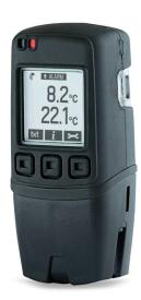
This standalone data logger measures and stores more than 250,000 temperature readings from two K, J or T-type thermocouple probes at a resolution of 0.1°C (0.2°F). It comes supplied with two K-type thermocouples capable of measuring from 0 to 200°C (32 to 392°F).
