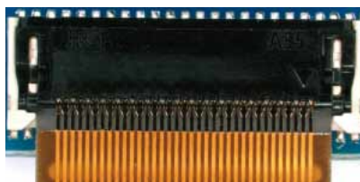
FPC is not inserted deep enough.
