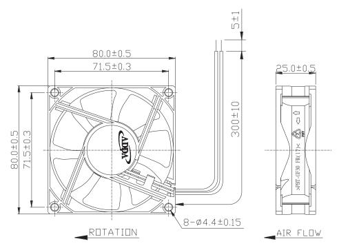
LEAD WIRES: UL 1007, AWG24, L = 300±10 mm
