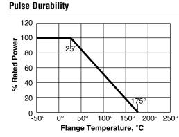
Limitation obtained by actual test with 0.01 duty continuous pulse repetition for TGHMV10R0JE, four times safety factor was considered. Please note this is not a specification, this is a typical data
