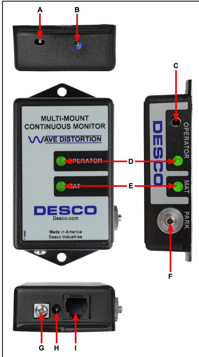
Figure 5. Multi-Mount Monitor features and components
