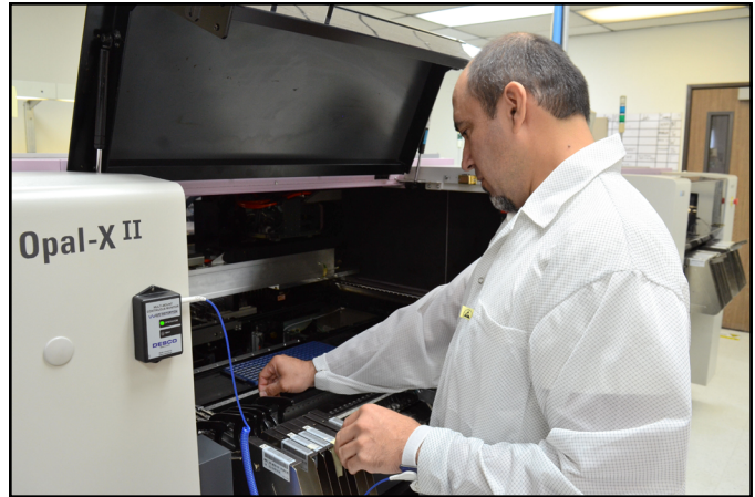
Figure 12. Using the Multi-Mount Monitor at a machine station
