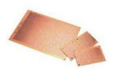
LARGE PCB BOARD Experimenters General Purpose Boards, Number of Holes: 2200, Dimensions:  $4\ 1/2\ x\ 6\ 1/4\ x\ 3/32$ , Applications: Assembling prototype, school and hobby projects, Features: Number markings for easy positioning
