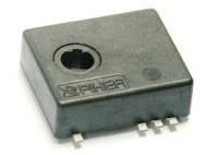
The MTS-360 provides a true breakthrough in contactless sensor technology by combining a through-shaft design with 360° absolute position feedback in an ultra miniature size. The result is the smallest fully featured rotary sensor on the market with reliability up to 50 million cycles.
