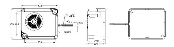
Dimensions : Millimetres Tolerance: ±0.5mm
