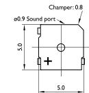
Dimensions : Millimetres Tolerance: ±0.5mm
