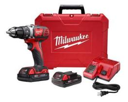
The most compact drill driver in its class is more powerful than the competition. Built with a Milwaukee® 4-Pole frameless motor, the M18<sup>™</sup> Compact 1/2" Drill Driver delivers 500 in-lbs of torque and up to 1,800 RPM. At only 7-1/4" length, this drill driver allows you access to the tightest work spaces. An all-metal gear case and 1/2" metal chuck provide maximum durability, even on the most challenging worksites. REDLINK<sup>™</sup> Intelligence provides
