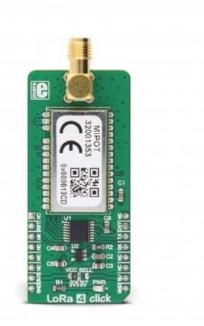
LoRa RF technology based transceiver
