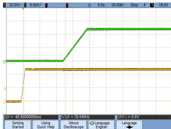
Figure 11. Vin Start-up Delay (CH2: Vout, CH1: Vin) (Vin=48V, Iout=50A, Cload=330µF, Ta=+25°C, 20mS/div)
