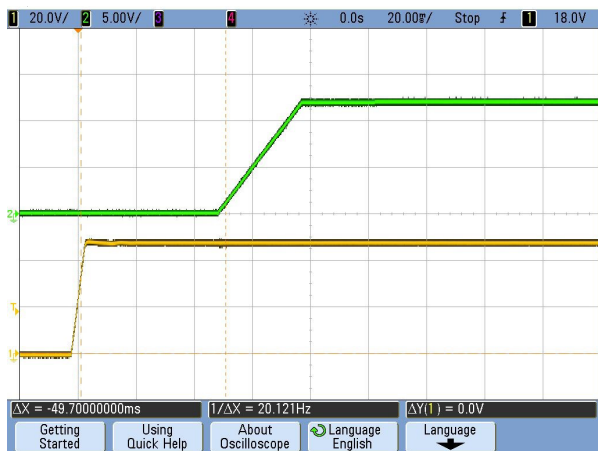
Figure 10. Vin Start-up Delay (CH2: Vout, CH1: Vin) (Vin=48V, Iout=0A, Cload=330µF, Ta=+25°C, 20mS/div)
