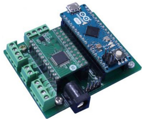
Figure 2. ONBB4AMGEVB Board with Arduino Micro and LV8714TASLDGEVB Board
