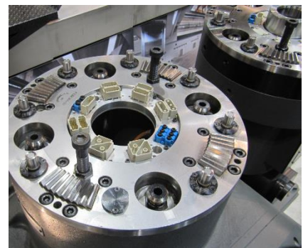
Exchange unit for quick and safe connection with pneumatic modules
