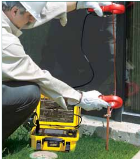
The Model 6471 performs a fast and easy way to measure the value of the earth/ground using the 2 Clamp method (no auxiliary rods needed).
