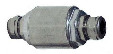
Heavy counterweight for use with MC series float switches. This metal counterweight is used to set or adjust the pivot point for the MC series of cable suspended float switches. The position on the cable relative to the switch can be used to adjust the liquid level differential between open and closed switch output. The MC series of cable suspended float switches from Cynergy3 are supplied with these counterweights.
