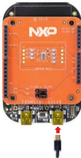
Figure 2: Connect board to computer
