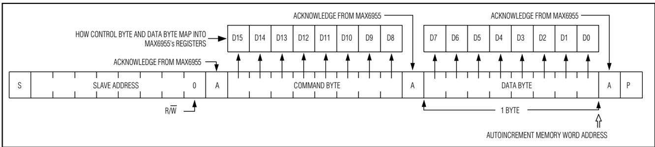
Figure 8. Command and Single Data Byte Received
