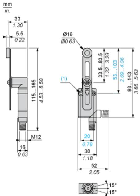
Mounting with Rotary Heads and Levers
