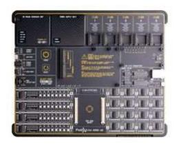
Development Board, Fusion Arm V8, On-Board WiFi Debugger, With MK64FN1M0VDC12 MCU Card
