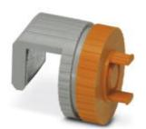
The optional holding device ensures the Rogowski coil is securely seated on busbars with a thickness of 10 ... 15 mm. During installation, the coil housing is pushed onto the flange of the holding device and snaps in automatically.
